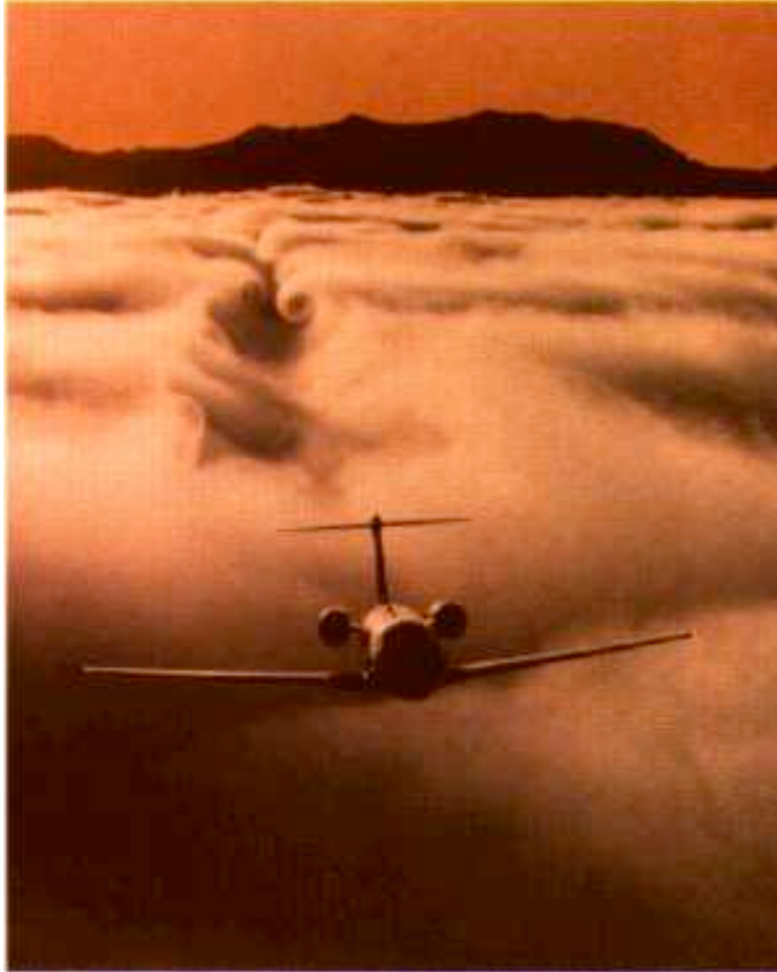
fig. 52 Wake vortex in the clouds far behind a jetliner.
