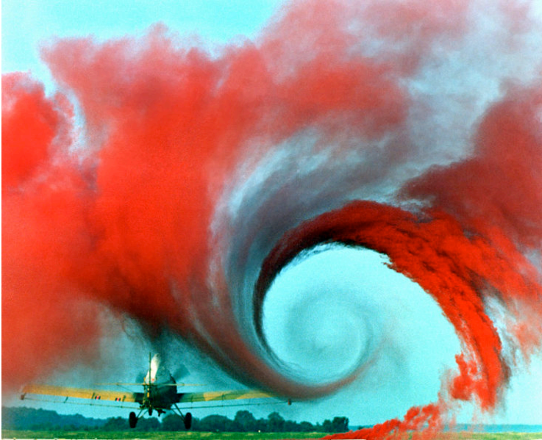
fig. 51 Wake vortex behind a crop duster.
